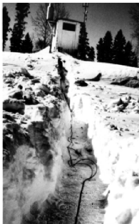
Figure 3. Ice motion detector sensor wires placed in slot in ice cover leading into gaugehouse.
