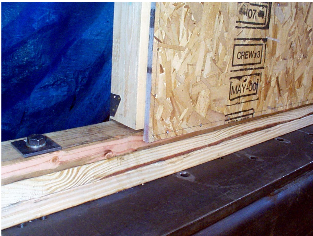
Figure 69. Stud lifting off of bottom plate in P3-6 monotonic test.
