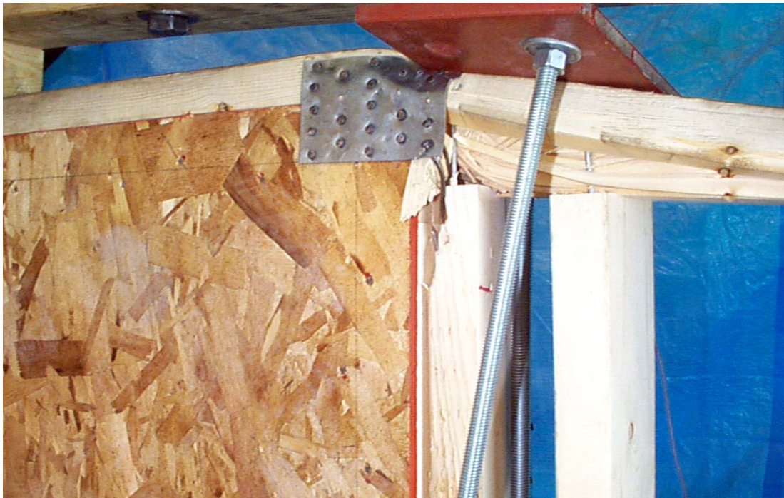
Figure 48. Torsion and bending in top plate.
