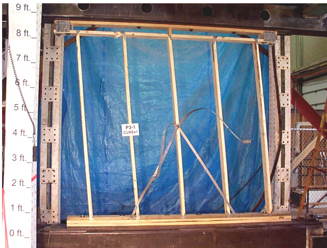
Figure 27. P3-1 CUREE1 panel strap failure showing straps still attached at the bottom and middle.
