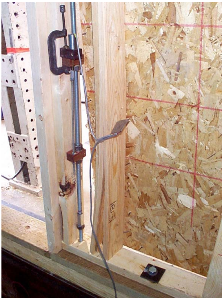
Figure 67. Back face corner of P3-3M panel showing stud cavity and threaded rod.
