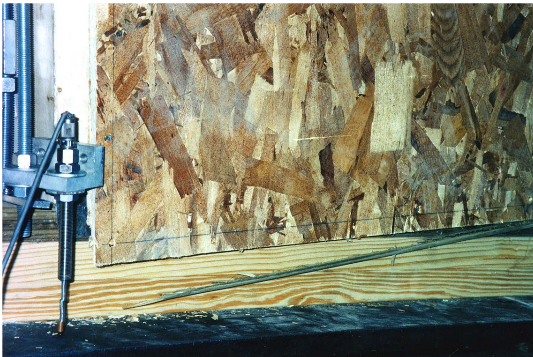
Figure 34. OSB pulling out of inset and crushing of hem-fir bottom plate.
