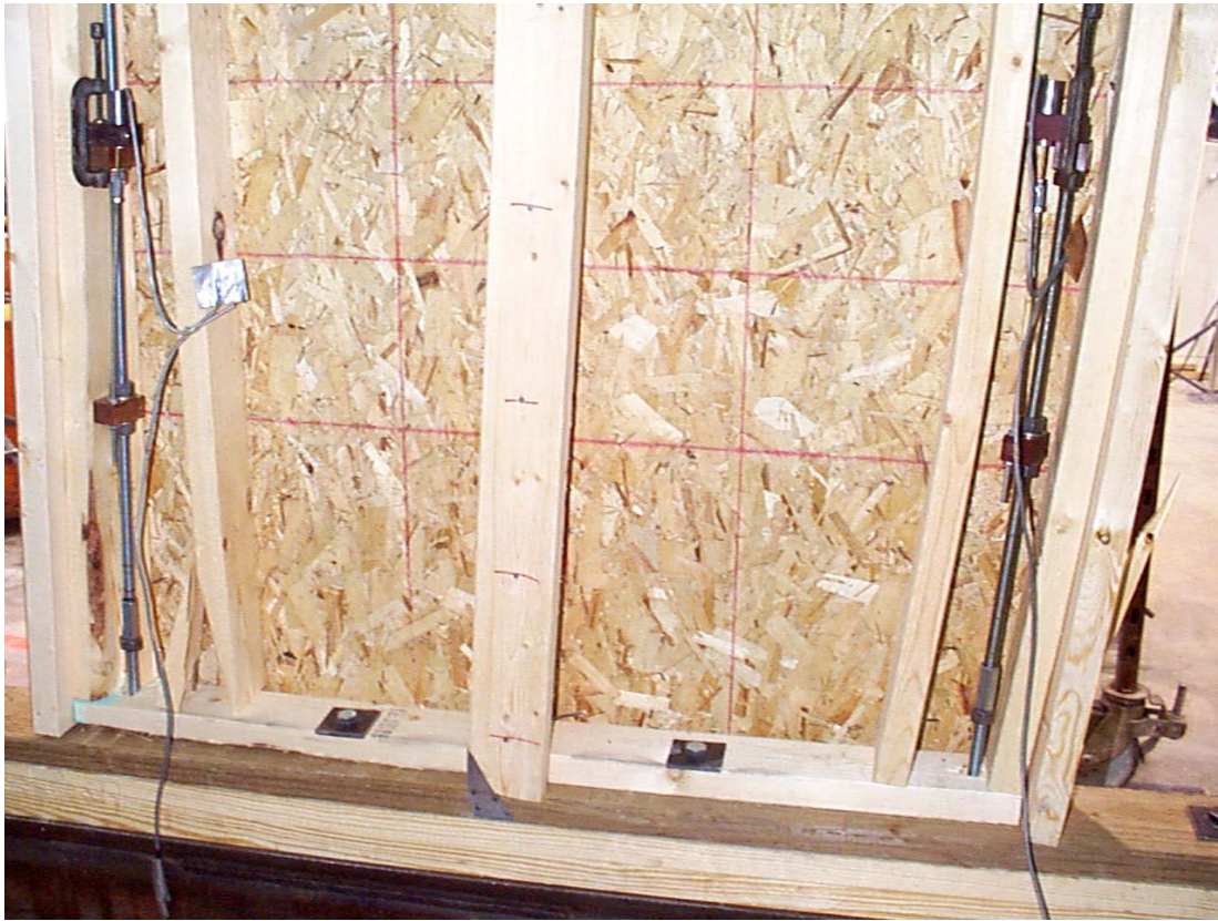
Figure 56. Interior face of P3-3M mono panel showing threaded rods.
