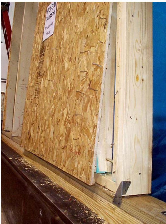
Figure 61. Stud to interior of the threaded rod cavity split in P3-3M CUREE1 test.
