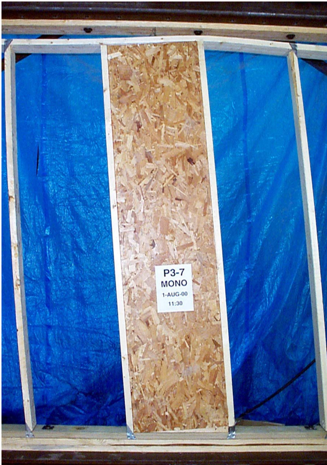
Figure 78. Overall view of damaged P3-7 mono panel at the end of test.
