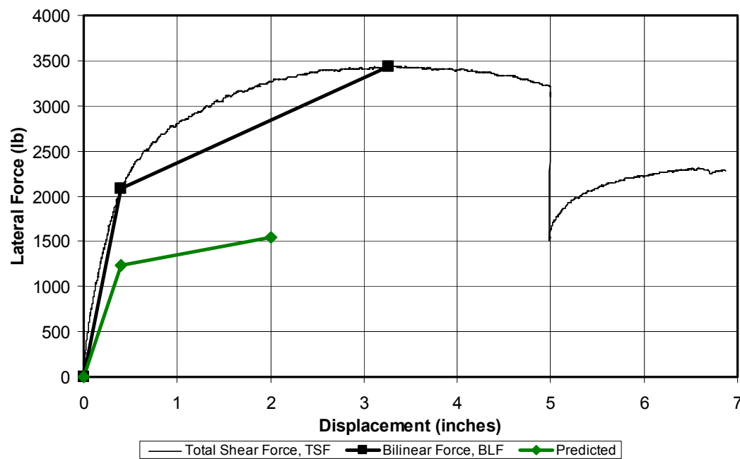
Figure 68. Lateral force (TSF) vs deflection for P3-6 monotonic panel.
