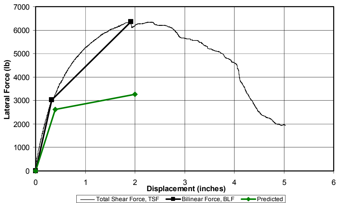
Figure 53. Lateral force (TSF) vs deflection for P3-3M monotonic panel.
