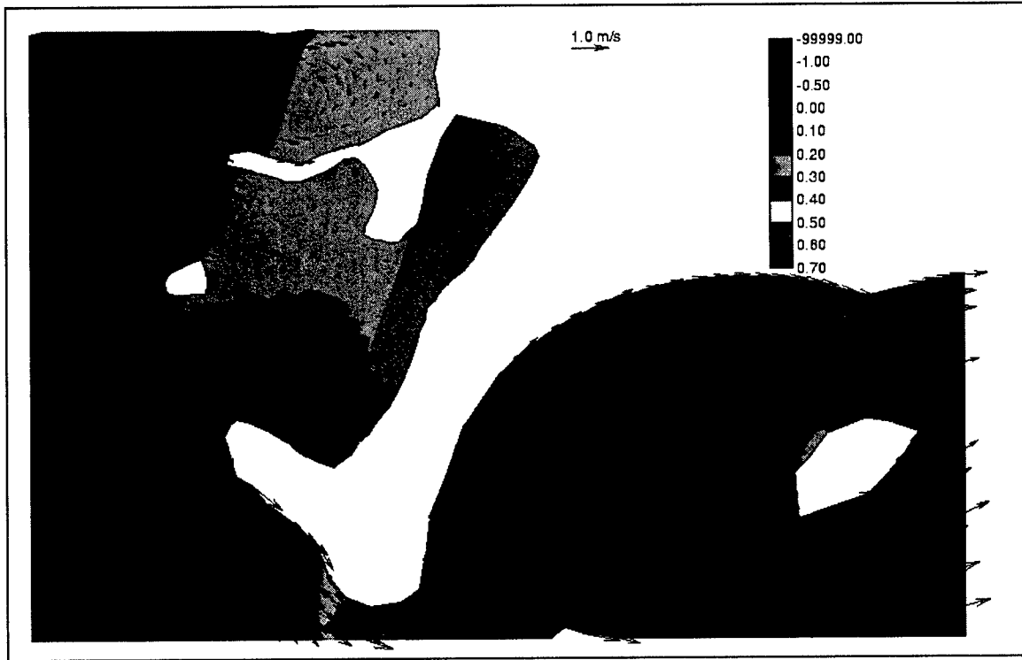
Figure 23. Post-expansion circulation vectors at Guayanilla for Hurricane Georges at day 3.28
