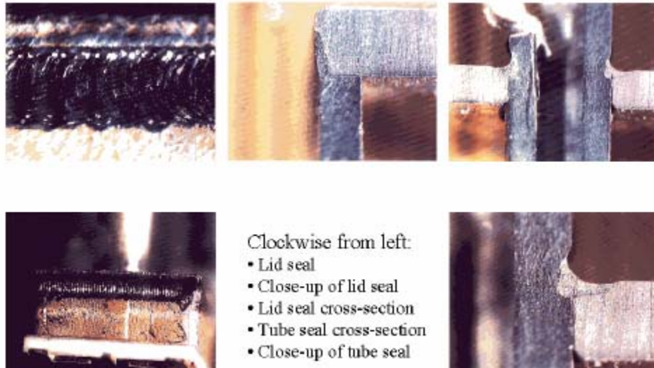
Figure 23. Welded Kyocera package, showing various close-ups of welds from the outside and in cross-section, showing penetration and weld extent. These welds were done using 2-3J pulses from a Unitek Miyachi Nd:YAG laser, at their facility in Monrovia, California.
