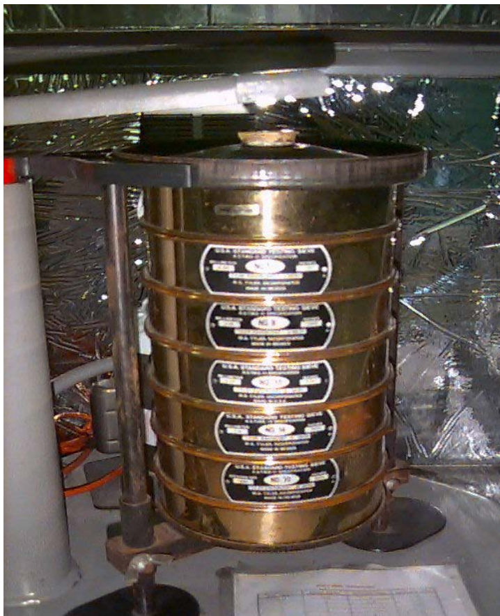
FIGURE 8. ROTAP SHAKER WITH 5 SIEVES IN PLACE.
