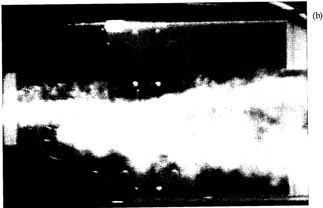
Figure 17. Flow-visualization images of a jet/vortex interaction. Circular jet, U_j = 1.2 m/s, contra-vortex jet, \theta = -90^\circ : (a) side view; (b) plan view.
