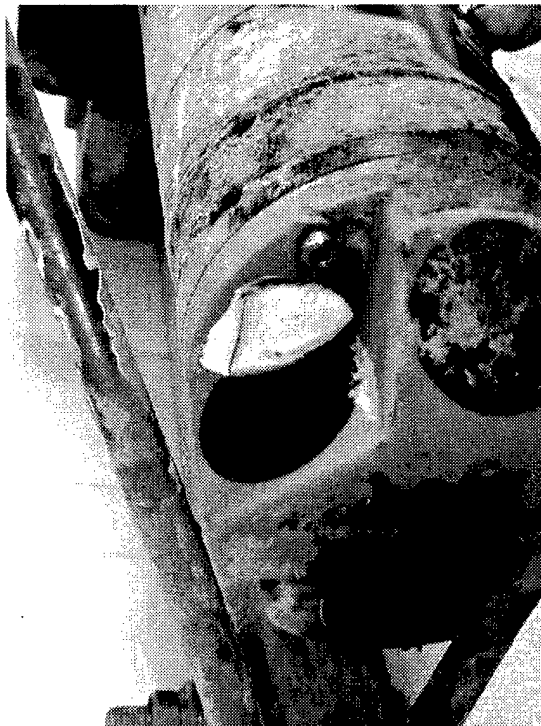
Figure 38. Fouling on the Aquadopp current meter.
