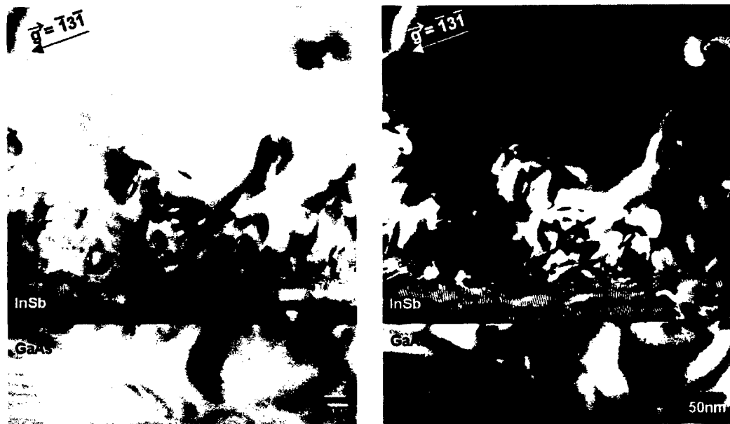
Fig. 18. TEM cross sectional images of GaSb overlayer grown on InSb/GaSb(LT) interlayer (a) bright field image and (b) dark field image (sample#3091400) exhibiting Moiré fringes at the GaAs/ InSb interface..
