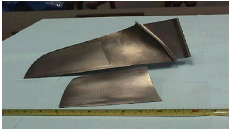
FIGURE 6.1.7.1 AFDS Integrated into a Fan Blade
