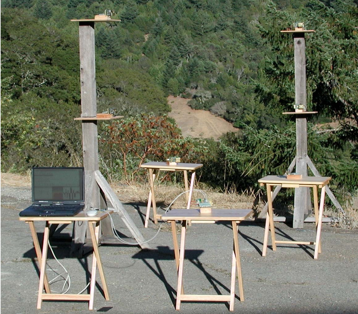
FIGURE 18. A group of seven networked Localizers, with one of them interfaced to a PC, is shown. The monitor program output can be seen on the PC screen. A wire-grid model for the environment for real time position display is shown on the left on the screen. A sample of the correlator output can be seen on the right. This network demonstrates the data flooding and cooperative networking concepts
