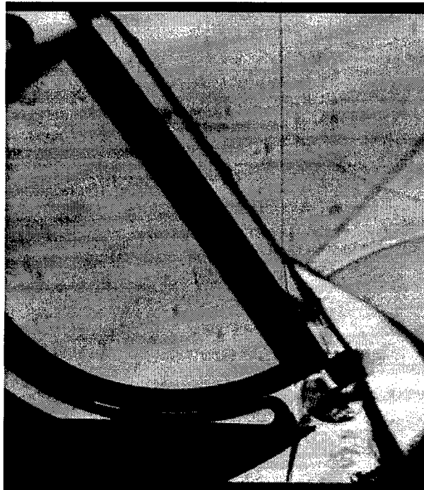
Figure A 3 Satin, M = 1.413 , \theta_w = 60^\circ , T = 1545\mu\text{s}
