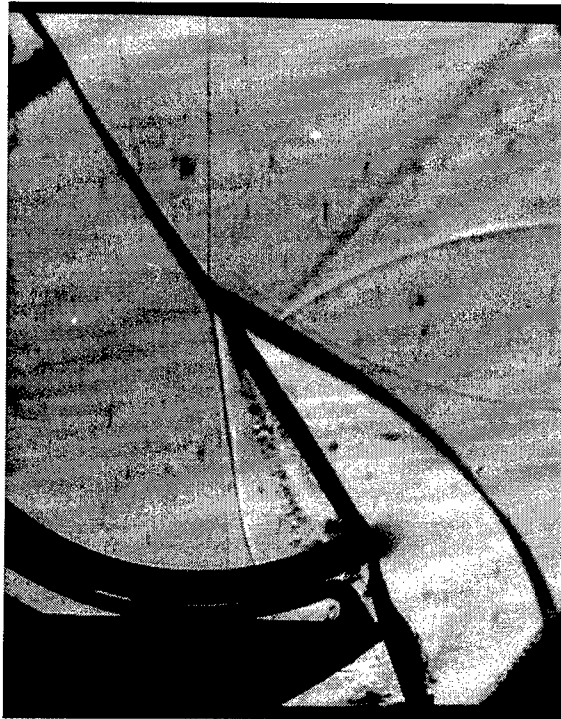
Figure A 20 Satin, No backing plate, M = 1.416 , \theta_w = 60^\circ , T = 1620\mu s
