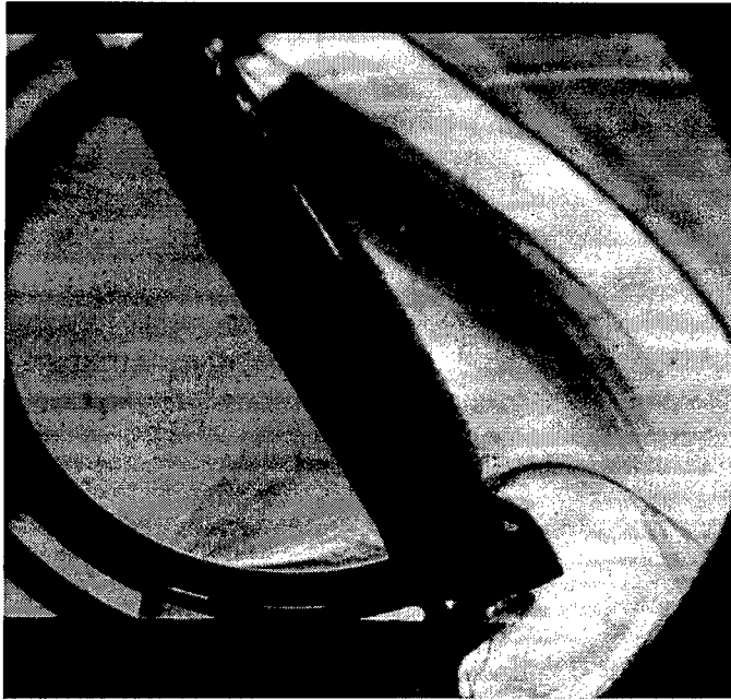
Figure A 6 Satin, M = 1.411 , \theta_w = 60^\circ , T = 1539\mu\text{s}
