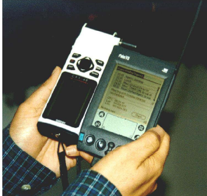
Figure 7: PDA (Palm VII) with GPS device for wireless, handheld communication between proxy and user.
