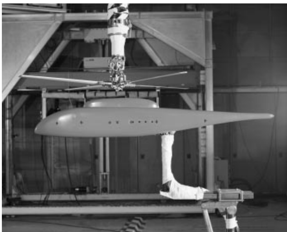
Figure 1. Photographs of the 2-meter Rotor Body INterference (ROBIN) configuration installed in the 14- by 22-Foot Subsonic Tunnel test section.
