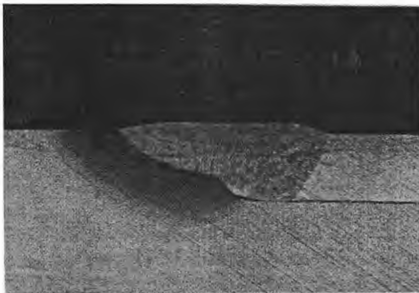
Figure 18. Cross section of a fillet weld specimen etched with 1% nital etchant; magnified 10 \times .
