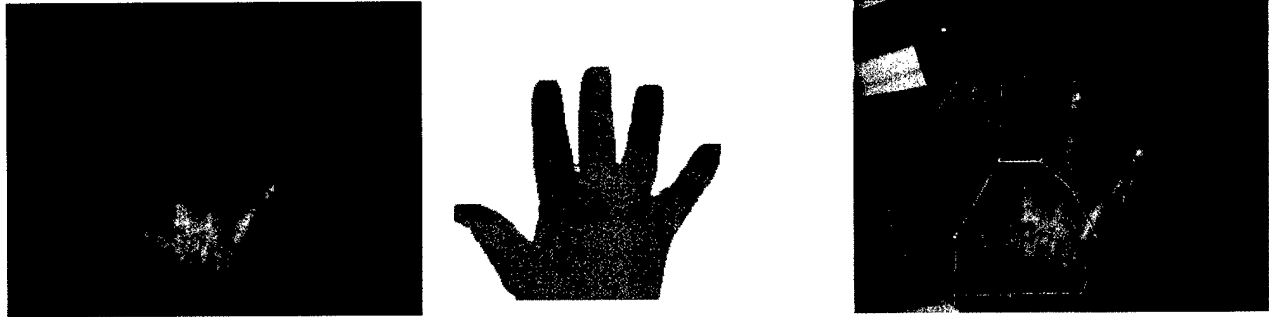
Figure 3: Illustration of image processing leading to hand and finger detection and labeling, skin color detection, skin region after expansion and contraction and labeling using the convex hull of the region as well as contour depth analysis.
