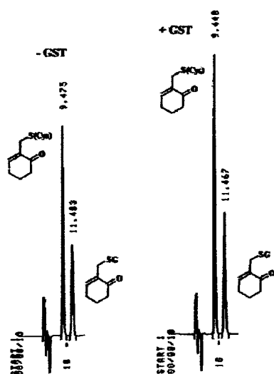
Figure 3. Fractionation of product mixtures in the absence and presence of GSTP1-1 by reverse-phase HPLC (Waters, \mu -Bondapak C 18 , 0.78 \times 30 cm).
