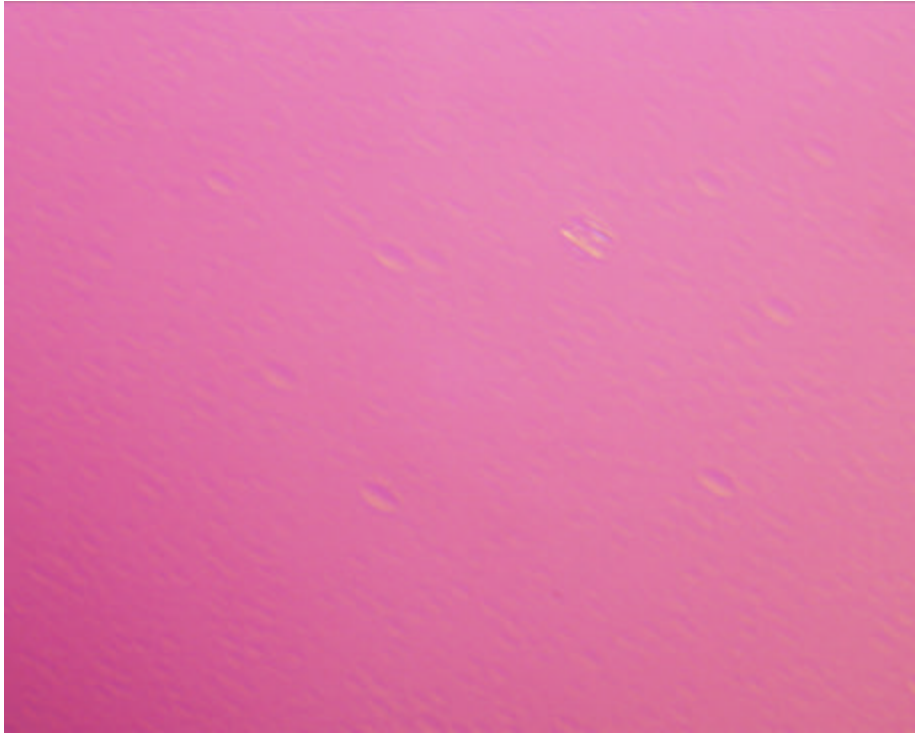
Figure 2. Nomarski photograph of a portion of the wafer shows the wafer surface morphology. The image was taken at 200X magnification.
