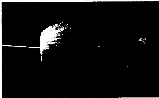
Figure 6 Fluoresceine injection from a tube located between the inner and outer shells. Ultraviolet lighting renders the streaklines visible. Transition is where the lines disappear.
