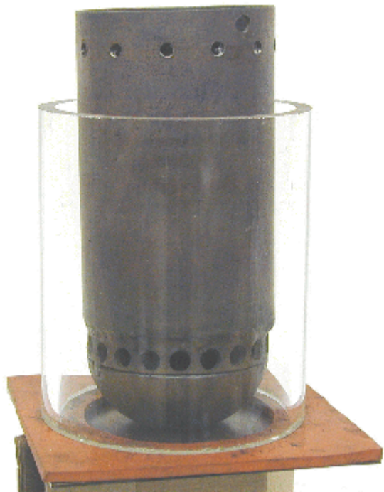
Figure C4. Stainless Steel, Wick, Vaporizing, Staged, Preheated Primary Air Burner
