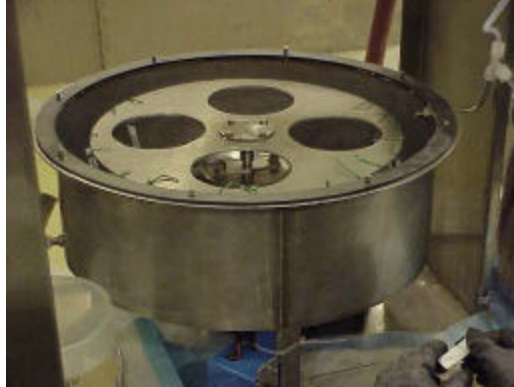
Figure 3.3 Exposure Chamber Showing the Carousel for Sampler Operation and Hanging Wires With Samplers Attached
