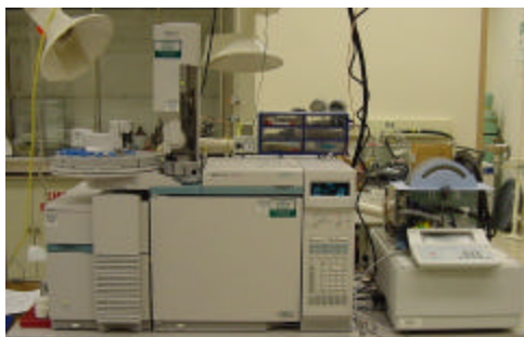
Figure 3.6 ATD-400 Attached To an HP 6890 GC with HP 5973 MSD
