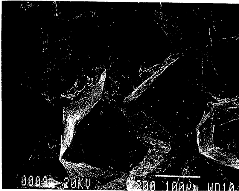
Figure D-2. Grains from the intergranular fracture surface of the failed strut mount (mag. 200 \times ).
