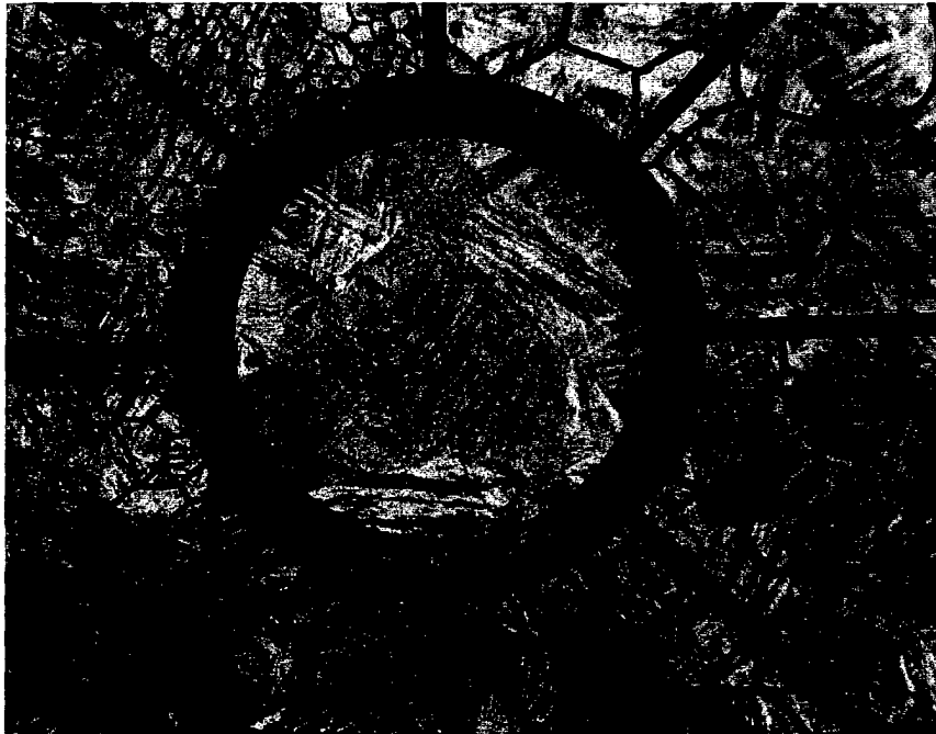
Figure D-1. Grain size of the failed strut mount with reticle overlay (mag. 100×).
