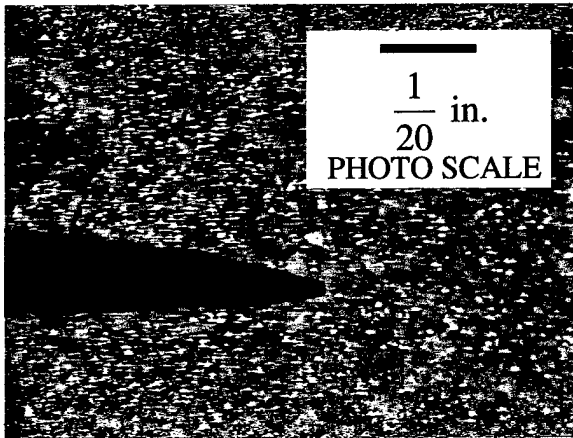
Figure 1. b = 1.0 in., Crack Tip Blunting
