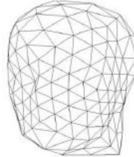
Fig. 2. Phase one - the surface S' obtained after the expansion and uniform re-sampling of the icosahedron of previous Fig. 1.
