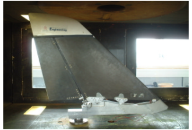
Figure 28. Wind tunnel and Fwd / Rear Attachment positions of the model
