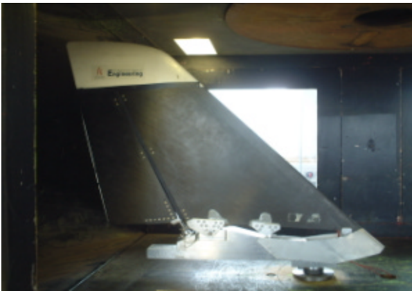
Figure 28. Wind tunnel and Fwd / Rear Attachment positions of the model
