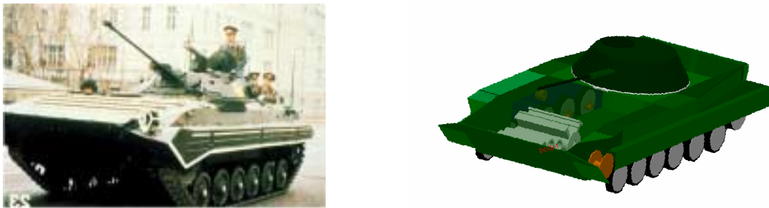
Figure 4. BMP-2 – Actual photo and in-progress DADS model.
