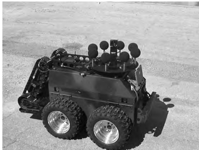
Figure 3. iRobot ATRV-2 with urban robot on dock.
