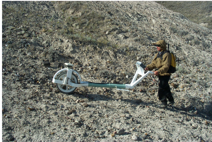
Fig. 2 – MTADS man-portable magnetometer system at the BBR
