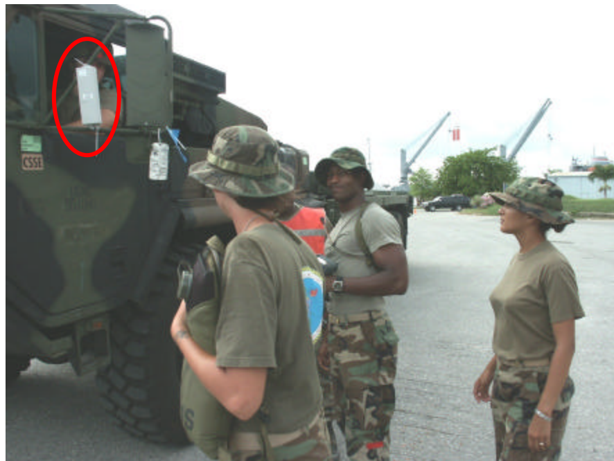
Figure 7: RFID Tag Placement
