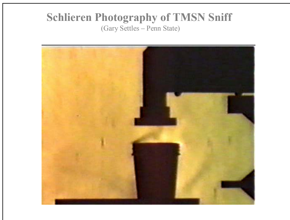
Fig. 7. Schlieren photograph/movie showing exhalation then inhalation of acetone vapor into the snout of TMSN-5.
