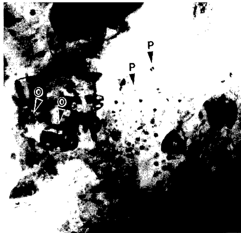
Fig. 8. TEM image of nanostructured Cr 3 C 2 -25(Ni20Cr) coatings exposed at 1073 K for 8h, "P" indicates precipitates, and "O" indicates matrix grains.
