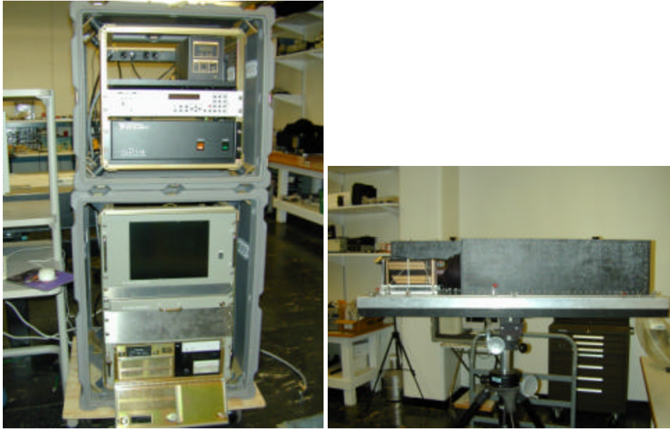
Figure 5.4. Pictures of LINUS. On the left side is the electronics section with the computer the amplifier and the camera pulser and cooler. On the right side is the optics section, which also includes the camera body and the scanner mirror assembly.
