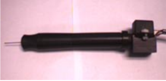
Fig. 1. Micron, the active error compensation microsurgical instrument
