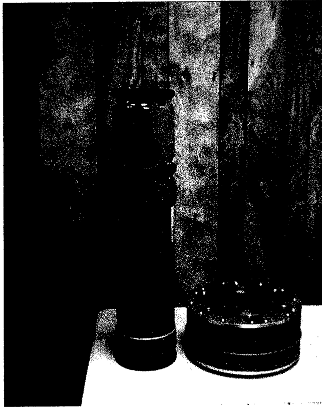
Figure 1. The LORAD LPX-160 and the rotating x-ray source collimator.
