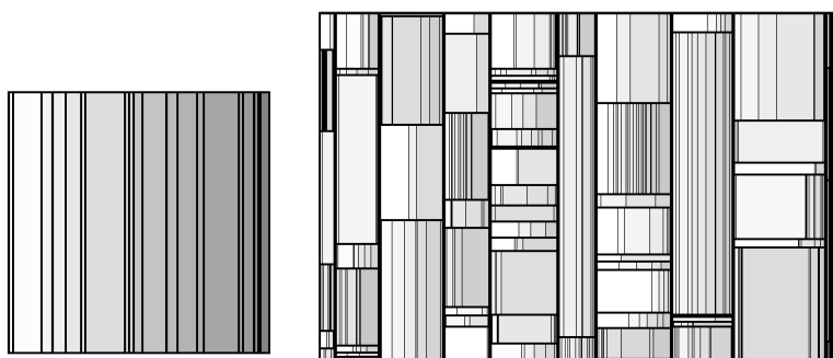
Fig. 1. The slice-and-dice treemap algorithm. Shading indicates order, which is preserved. The left image shows a single level treemap, and the right image shows a hierarchical application of the same algorithm.
