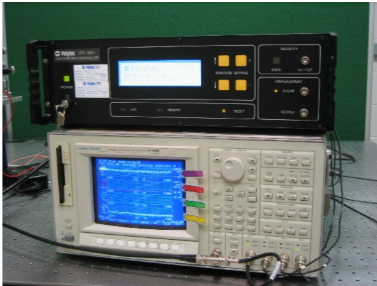
Figure B.4. Polytech OFV-3001 Controller(top) and Onisoki FFT Analyzer with Signal Generator(bottom).
