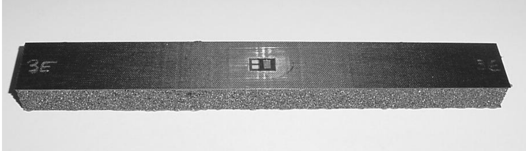
Figure 3.5 Prepared Specimen With Attached Strain Gage (Specimen 9)
