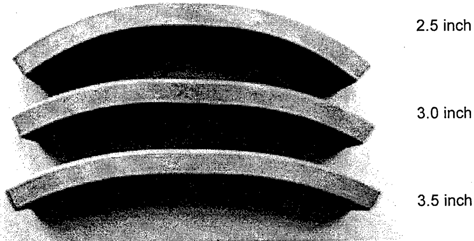
Fig. 14. Results of de-coiling samples with different radius of curvature and constant thickness.
