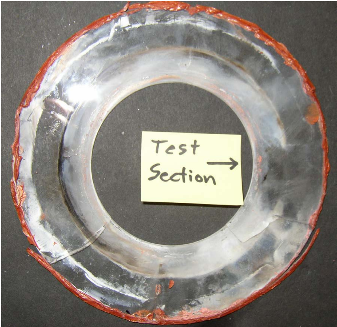
Figure 13: Quartz Window Picture Following Testing
