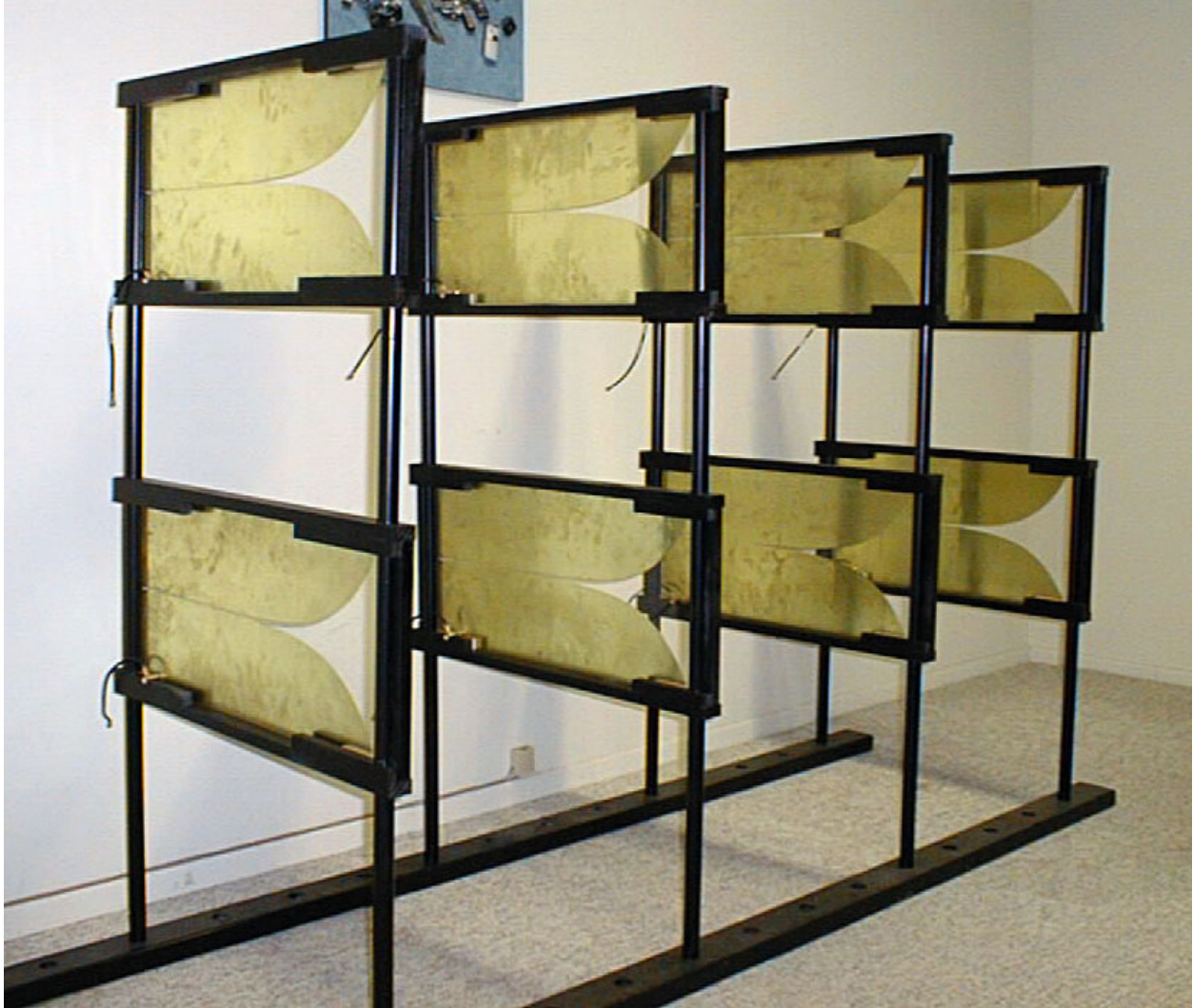
Figure 17 - Experimental antenna array.
