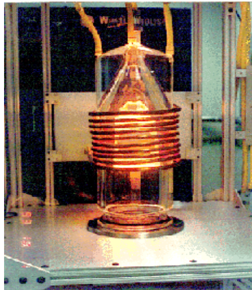
Figure 2.20: Ambient pressure chemical vapor deposition reaction chamber [2]
