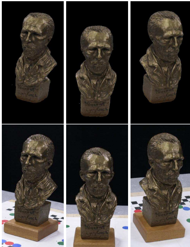
Figure 18: Synthetic images using the estimated radiance tensor (top) compared with the true images taken from the same vantage point.
