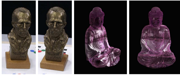
Figure 16: Scenes with strong specularities (left) or made of translucent materials with no distinct point features are a challenge to most stereo algorithms.
