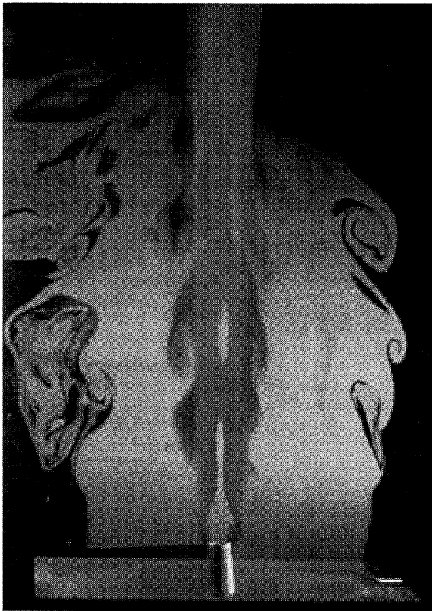
Figure 4. Flow visualization of driven-vortex hydrogen jet diffusion flame.
