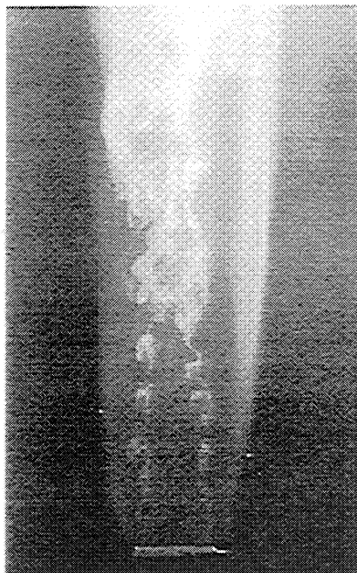
2D Laser sheet visualization
