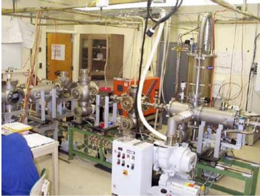
Figure 11. Molecular beam apparatus for measuring the magnetic properties of atomic clusters.
