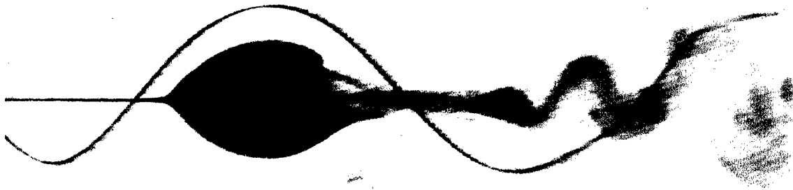
Figure 3-23: Dye visualization of breakdown in pipe flow ( ref. 23 )
