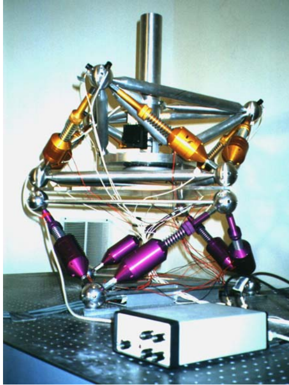
Figure 3: The top hexapod performs fault tolerant, high precision pointing and tracking. The lower hexapod induces high fidelity 6 axis vibrations matching candidate applications.
