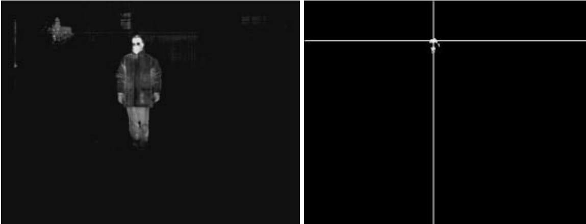
Figure 2. Examples of typical images. The image on the left is an example of raw image data collected from one of the infrared cameras viewing the test subject. The image on the right is an example of a binary image, where the object (subject's head) has been selected and its centroid marked.
