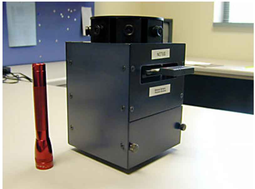
Figure 3. Packaged sensor module. 4 CMOS cameras are distributed across the top of the module.
