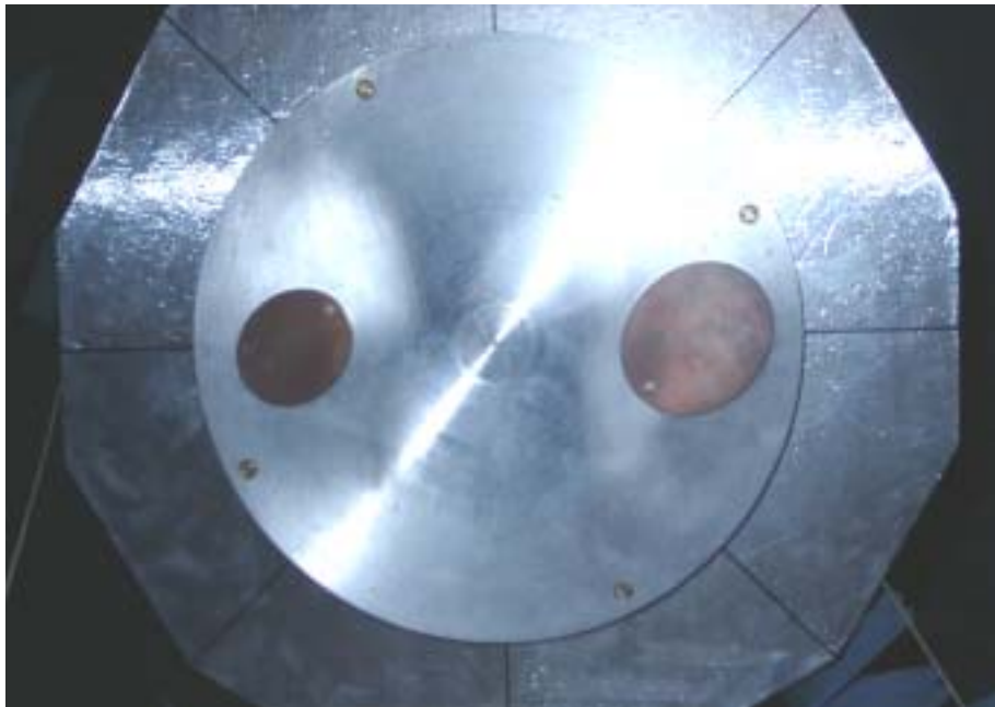
Figure 4. Patch Antennas and Ground Plane
