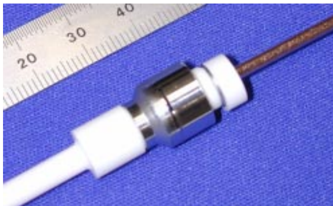
Figure 29. Close-up of Feed-Through
