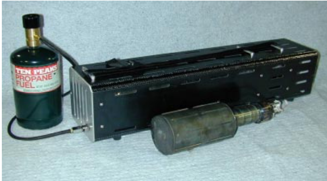
Figure 42. Generator with GF-2B Converter
