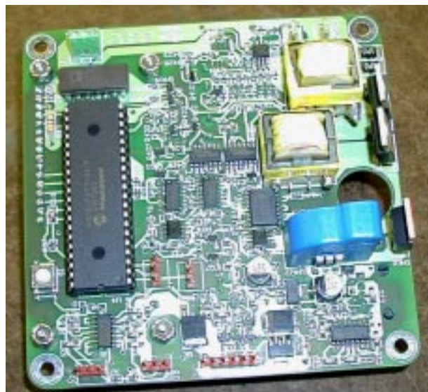
Figure 38. Back Side of Control/Power Board
