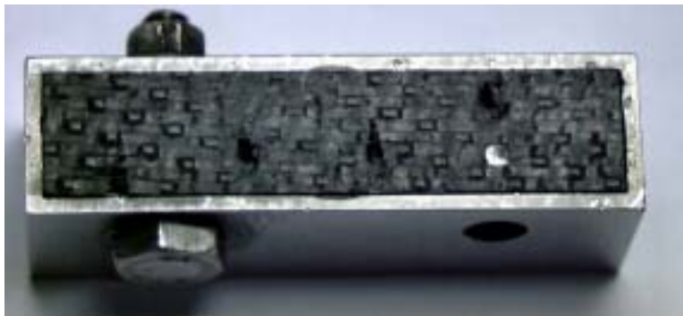
Figure 1. Example of a Carbon-Phenolic Sample in the Test Holder
