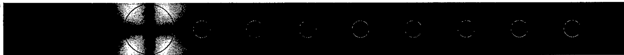
A bound state on the surface of a square-lattice PC in which the first rod is enlarged (one period in the vertical direction is shown).
